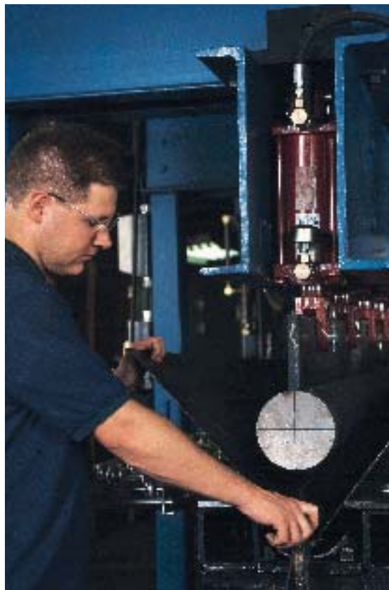
With the guidance of CEAT professors Richard Lowery and Larry Hoberock, OSU undergraduates developed an innovative and inexpensive method for the fabrication of tapered steel poles. Mechanical engineering senior Pat Straughan, above, makes adjustments to the prototype.
