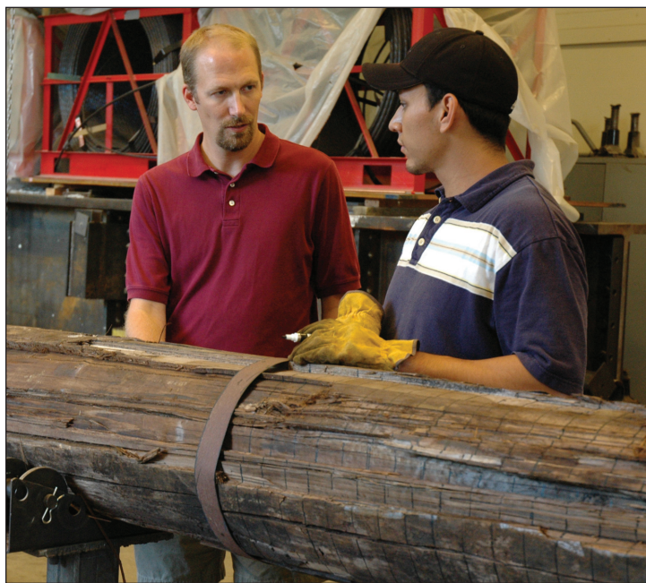
Research by civil engineering associate professor Robert Emerson (left) on cost effective techniques to evaluate bridge-supporting timber piles is a study at OSU for the Oklahoma Transportation Center.
