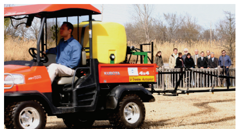
Brazilian visitors watch OSUIT precision agriculture instructor Carlos Augusto drive a KUBOTA RTV equipped with a GPS-based auto guidance system and variable rate sprayer programmed to apply amounts of material in the exact correct spot on the ground to maximize crop growth and profit.
